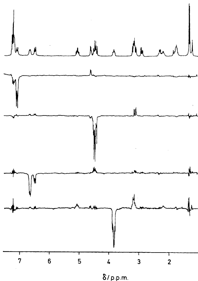
Figure 1. In the top trace the off-resonance 270 MHz 1 H n.m.r. spectrum of [Ala 4 ]-desdimethylchlamydocin in CDCl 3 is shown; the lower traces refer to difference spectra. Negative peaks result from the irradiated proton; positive peaks are due to the homonuclear Overhauser enhancements (n.o.e.) discussed in the text.
